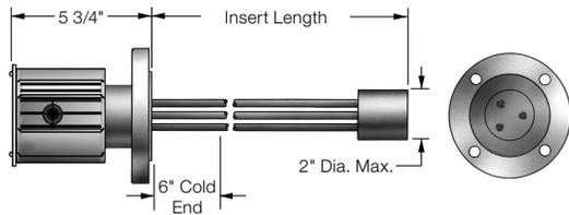
Figure 36 – 3" - 150 lb Flange (Three Straight Elements)
