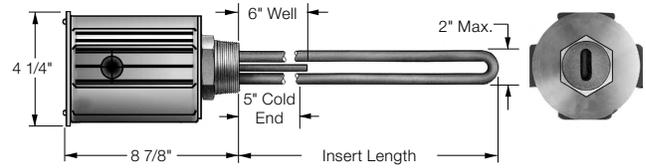
Figure 37 – 2" NPT Screwplug (One Hairpin Element)
